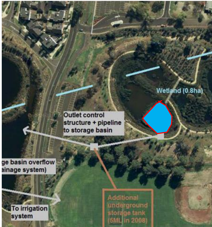
Fig. Schematic overview of Royal Park stormwater wetland and reuse system (City of Melbourne, 2013)
